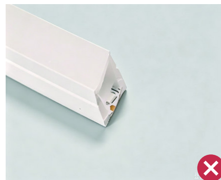
Incorrect: uneven cut. Keep the PCB flat.
