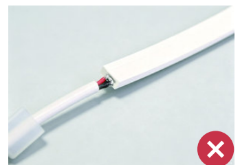
Incorrect: solder burr
