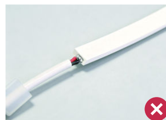
Incorrect: solder burr. Avoid shorts and bridges.
