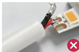
Incorrect: poor joint. Inspect joint strength.
