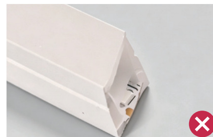
Incorrect: uneven cut. Keep the PCB flat.
