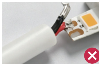
Incorrect: poor joint. Inspect joint strength.
