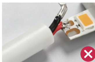
Incorrect: poor joint. Inspect joint strength.
